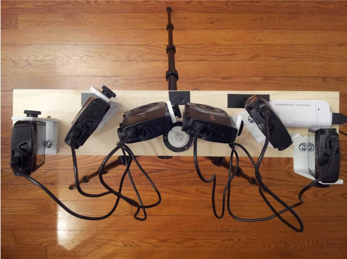
The board measures about 18 x 3.5 inches, and weighs a little less than a pound. With all of the cameras, cables and other hardware attached, the total weight is about 3 pounds, about a pound lighter than a Nikon D800 DSLR and Nikon 14-24 lens. Because the array is quite light, it doesn't require a particularly sturdy tripod. I have been using mine with a small Slik Compact XL tripod.
